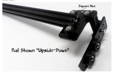
3. Flip main rail so it's "right side up" and attach headboard using 2x M5 screws and washers. Do not tighten them yet, we'll need to align front rollers to back rollers.
