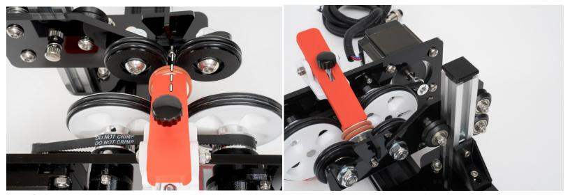
Once it's aligned, secure M5 screws, but DO NOT OVERTIGHTEN them or you might crack acrylic!
