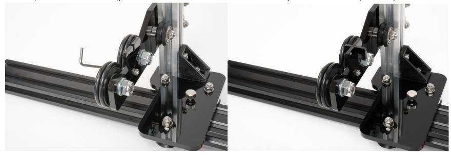
4. Attach headboard to the main rail using 2x M5 screws and washers. Do not tighten them yet, we'll need to align front wheels to back rollers.
