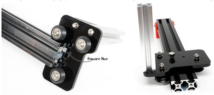
2. Install **footboard** on the **vertical post** of **carriage**. Place as shown on images below. Slide in large **square nut** into rail slot and slide in 3 **v-wheels** into grooves as shown. Insert plastic **cap** on the end of the **vertical beam**.
